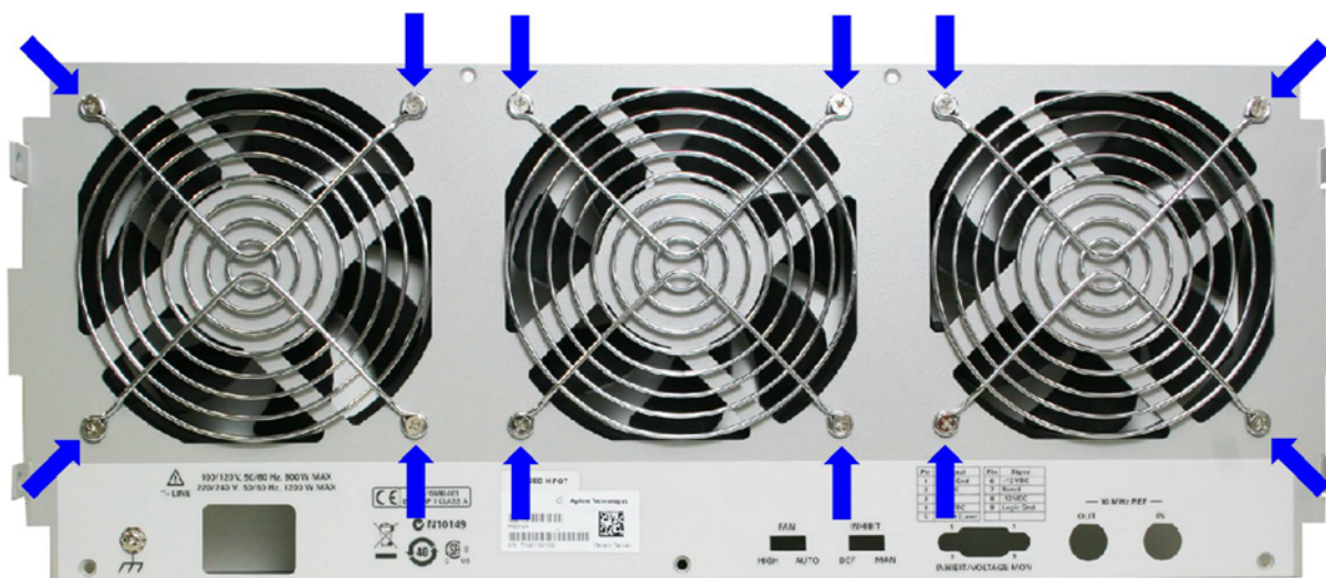
Figure 80 Remove these screws to detach the fan assembly
