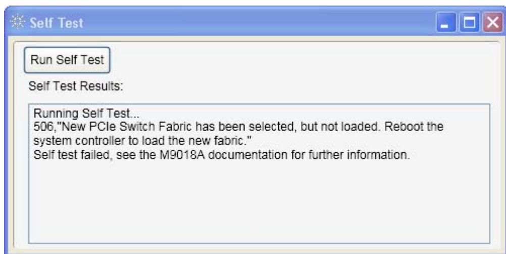
Figure 46 If self test is run prior to rebooting your computer, it will detect that the computer needs to be rebooted
