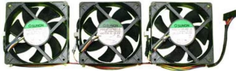
Figure 81 The fan assembly prior to mating with the rear panel
