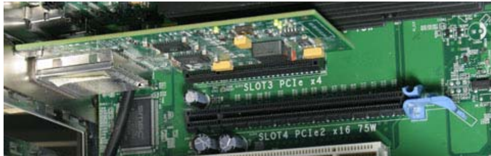
Figure 60 An example PC’s x8 (x4 mode) and x16 (x16 mode) PCIe slots
